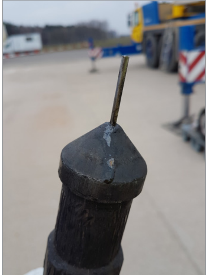
A timed clean cut was made on the wire within inches of the toolstring, on the first run in the hole.
